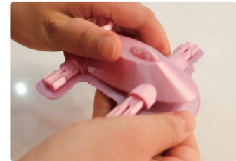
Remove support material
